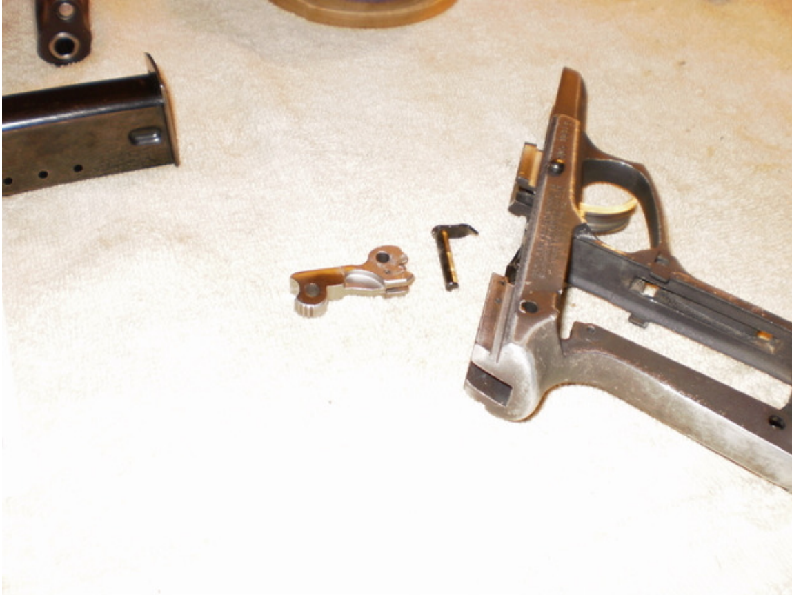
Hammer & Pivot Pin Removed
