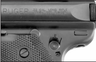
Figure 1. Safety in the “off” or “fire” (F) position. Safety is all the way down .
