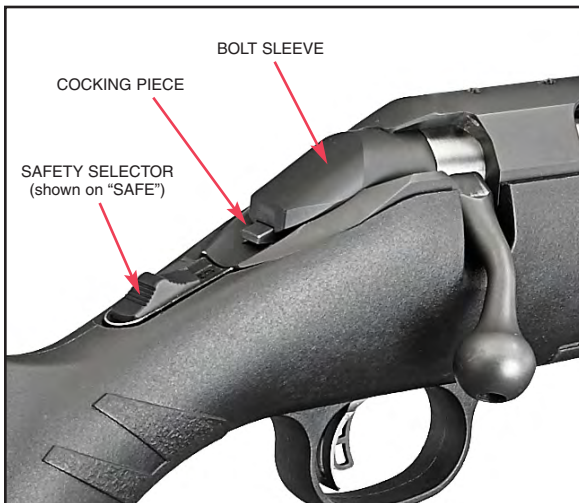
Figure 2. In this photograph the cocking piece is shown cocked (protruding from the rear of the bolt sleeve). (The safety selector should be in the "Safe" position when the bolt is being removed or installed.)
