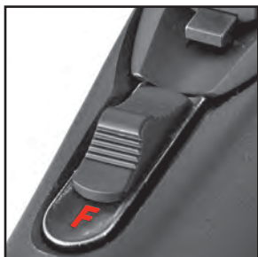
Figure 5. Safety selector in “FIRE” (full forward) position. The safety selector should be moved to this position only when the gun user is actually firing the rifle. When the safety selector is in the fire position, it is referred to as being “off.” (When the safety is in the “SAFE” position, it is referred to as being “on.”)
