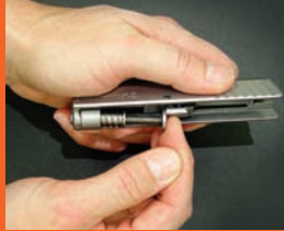
Press guide rod assembly releasing it from barrel
