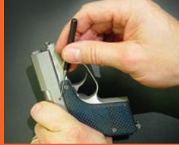
Move slide back locating barrel pin.
