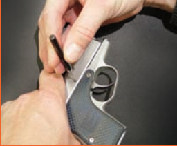
Turn over and, using a 1/16 pin. Push out the 5/32 barrel pin.
