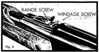
The receiver is designed with two dovetail grooves cut into the top panel for attaching the "tip-off" type of telescope mount (Fig. 3). The mount may be easily slipped into receiver grooves and tightened in desired position.
