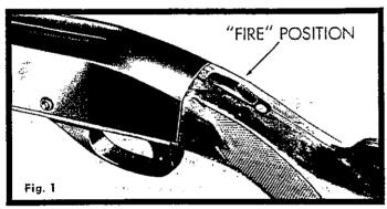
FIRE — Push safety forward to FIRE position (Fig. 1). RED indicator button will show to rear of safety in FIRE position. Pull trigger to fire each round loaded into barrel. After firing, the autoloading action is designed to cock the rifle after the fired cartridge case is ejected.
