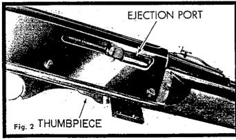
TO LOAD MAGAZINE — Clip magazine may be removed by depressing rear of magazine latch thumbpiece (Fig. 2) and pulling clip from bottom of rifle. Load cartridges into magazine. Capacity of magazine is ten (10) cartridges. To reassemble, fit channel opening on back of magazine over end of magazine guide. Push magazine upward until locked in place by magazine latch.
