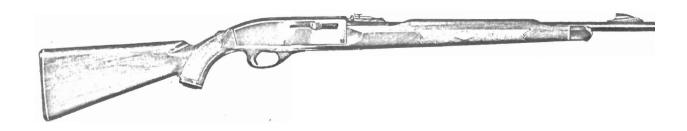
SAFETY PRECAUTIONS BEFORE HANDLING OR SHIPPING. With empty Magazine Tube locked properly to rifle, pull Bolt Handle repeatedly. This should eject any live rounds left in the action or in the Magazine Tube. Then check cartridge chamber in Barrel for a live round.
