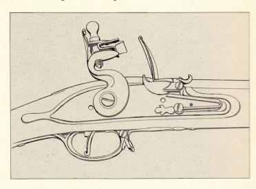
(ii) Put the lock on half cock and close the pan cover. Blowing down the barrel at this stage will help you to ascertain that touch hole is free. If you cannot blow down the barrel there are two possibilities: (a) the touch hole may be blocked, in which case clean it with a pin or piece of wire, or (b) the weapon may be loaded. If the latter, find our immediately why this should be the case and resolve never ever to let it happen again.
