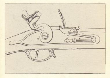
Flints: The flint is a vital part of the weapon and should be kept in good condition and replaced when necessary. It is held in position between the jaws of the cock with a small oblong of leather round it. This also helps to protect the top jaw screw from the back edge of the flint. The flint is normally placed with its longer flat face uppermost, but we suggest that you experiment to find the position of the flint which will give the most satisfactory spark consistently.
