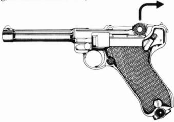
The magazine follower button will activate the last round stop and the action will stay open. (If it doesn't, something is wrong.) You can then remove the magazine and the action will stay open as shown here. Make sure the safety lever is on 'Safe'.
