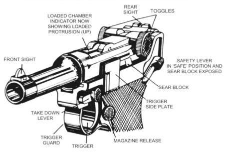
In doing so, the toggle assembly will snap forward, strip the top cartridge out of the magazine and load it into the chamber. You are now holding a loaded pistol with the safety "ON" and a round in the chamber! Take note of the loaded chamber indicator and see how it protrudes above the surface of the breech bolt. Keep the pistol pointed 'Down-Range' at all times.
