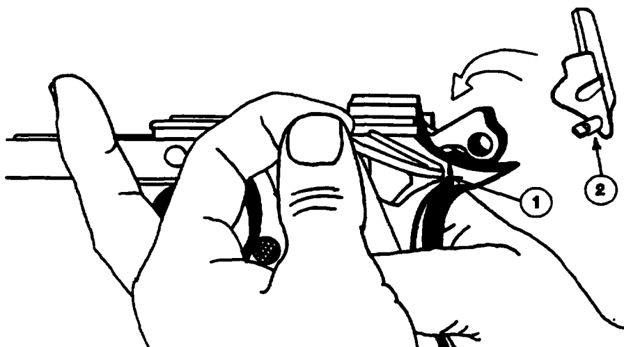
Figure 6-21. Removing Ambidextrous Thumb Safety
