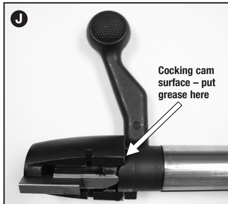
Put a small amount of grease on the cocking cam surface
