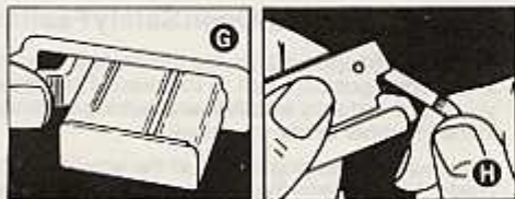
Releasing the clip magazine
