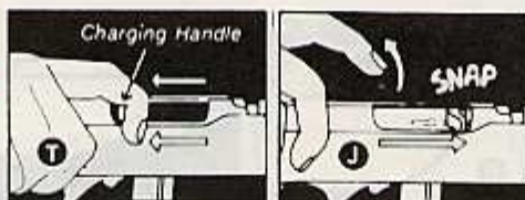
Pull charging handle all the way back
