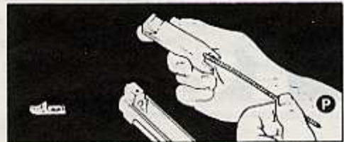
Remove charging handle, recoil spring, and spring guide
