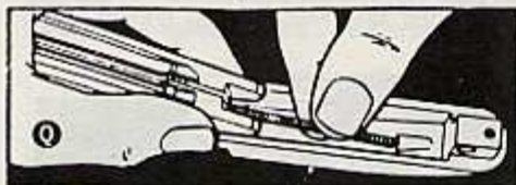
Support recoil spring to prevent kinking
