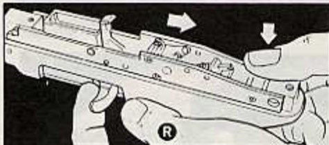
Pull charging handle back to replace action
