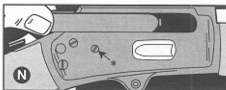
Replacing breech bolt (*Keep this screw tight)
