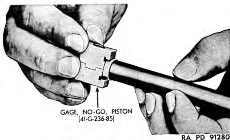
Figure 35. Gaging diameter of piston.
