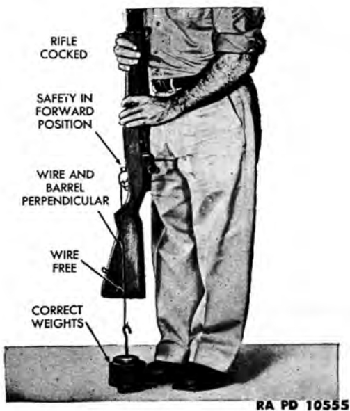
Figure 4. Checking trigger pull with weights.
