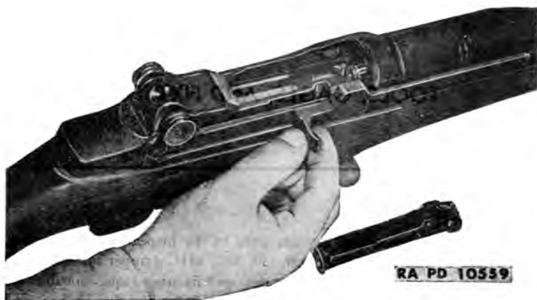
Figure 7. Checking headspace with field test bolt and headspace gage.
