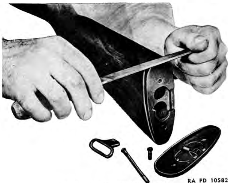
Figure 74. Fitting butt plate on stock.
