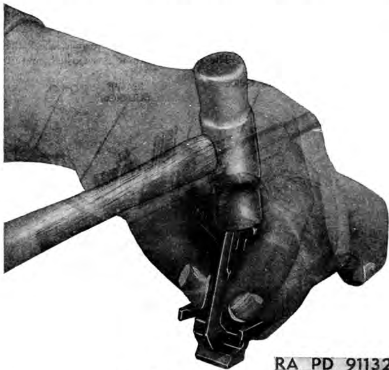
Figure 58. Installing follower slide.
