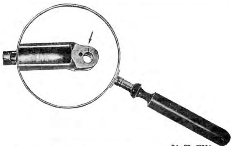
Figure 65. Hammer spring housing—important points to be inspected.
