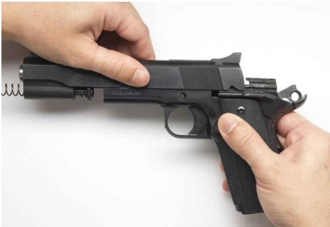
Fig. 7 Remove the Slide
