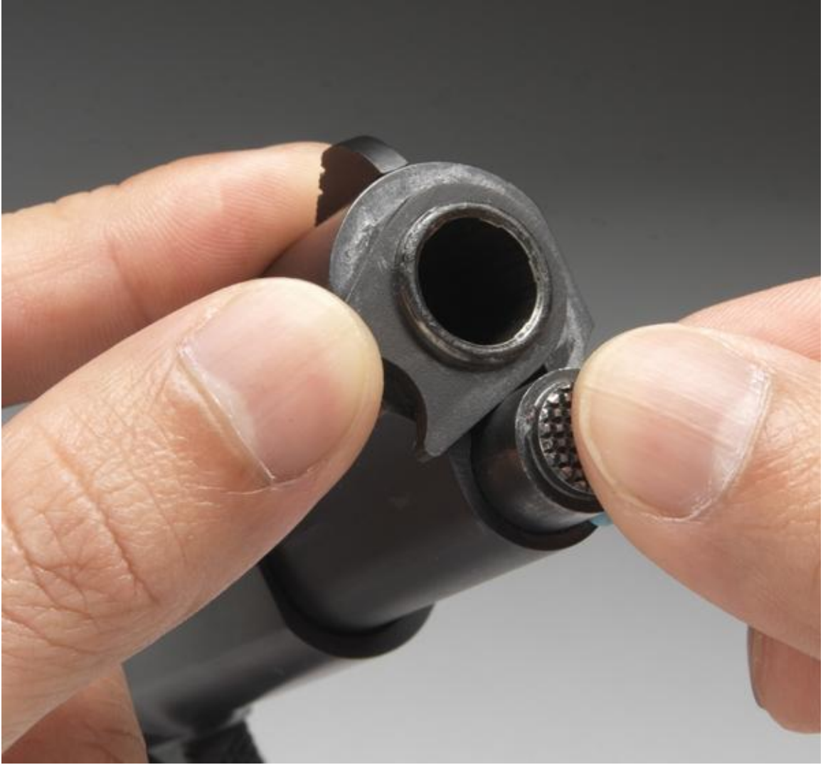
Figure 5. Remove the Recoil Spring Plug
