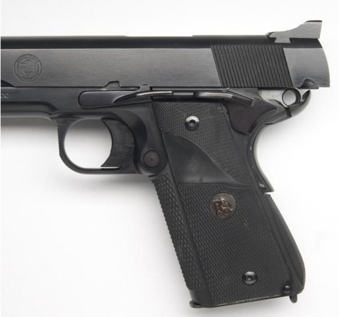
Fig. 6 Move Slide to the Slide Stop Disassembly Notch
