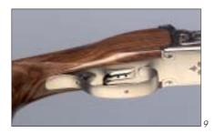
To adjust the trigger position, loosen the screw about one turn with the hex key provided (See image). The forward opening in the trigger is where the screw is. The rear opening does not contain anything. Slide the key to the desired position and gently retighten the trigger position screw.
