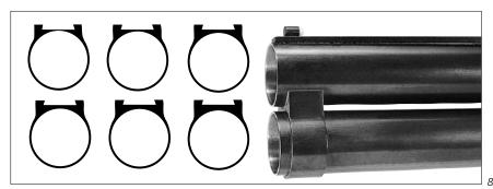
The point of impact of the bottom barrel of the K-80 and K-20 can be raised or lowered in relation to that of the top barrel simply by changing the front barrel hanger No. 606. The hangers have dovetails of varying width which change the height of the bottom barrel. (See illus. No. 8). If you wish to have the bottom barrel pattern higher, select a ring which is thinner at the dovetail. A thicker ring will move the pattern lower.
