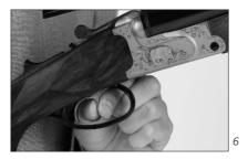
After you made sure that the gun is uncocked, put your thumb behind the trigger and keep slight pressure against the trigger. Then lay your index finger of the same hand against the front of the trigger, but still maintain at the same time slight thumb pressure from behind. Now move the trigger slightly in the pull direction until it disengages from the hair trigger setting holding the trigger firmly between the two fingers the whole time.
