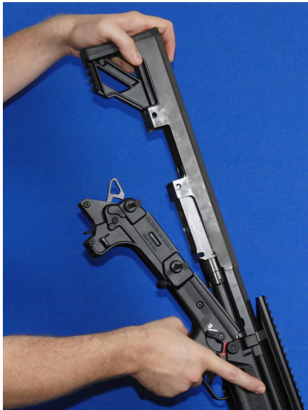
Figure 34: When the action is opened, pull the top cover off
