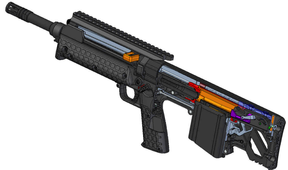
Figure 8: The charging handle is fully to the rear and ready to be released
