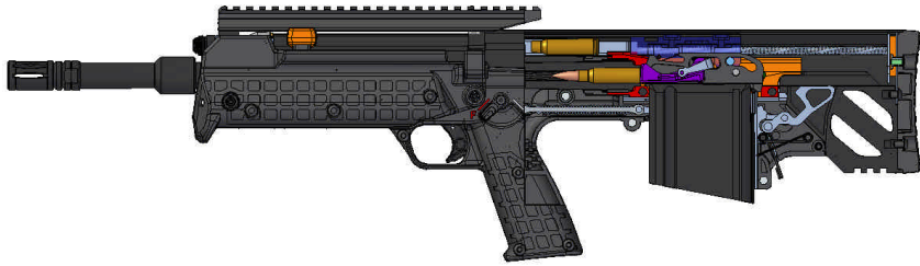
Figure 21: The extractors are down, the hammer is cocked, and the rifle is again ready to fire.
