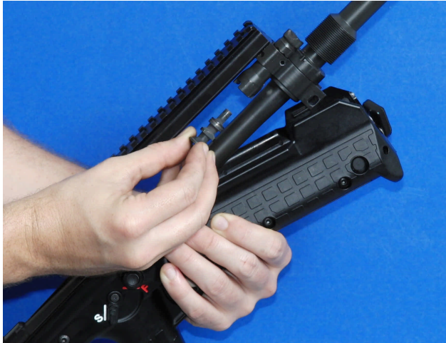
Figure 48: Wiggle the piston to remove
