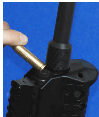
Figure 28: Using the rime of a cartridge to turn the gas restrictor cap
