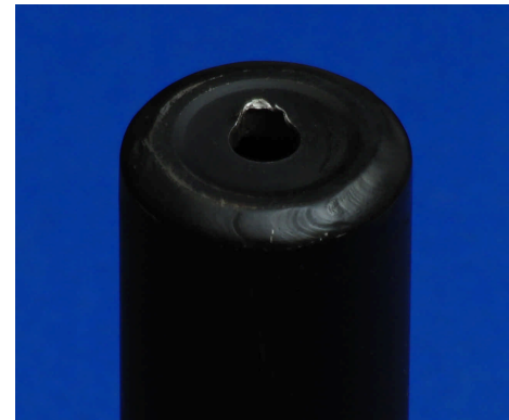
Figure 2: Baffle Strike caused by Subsonic Ammo
