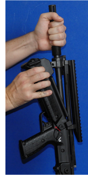
Figure 39: Grasp the barrel with one hand and pull down the handguard
