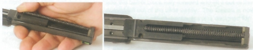
Snapping the captive recoil springs in place
