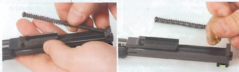
Removing the recoil spring assembly and the buffer
