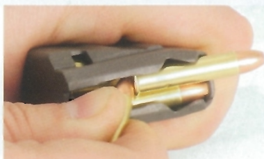
Unloading the magazine by pushing rounds forward
