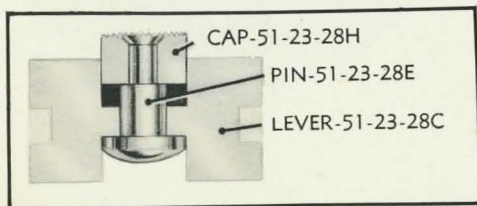
Figure 9—Lever, Breechblock, Assembly
