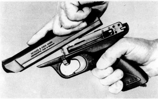
Fig. 7: Removing the slide Quitar la corredera Enlever le bloc-culasse
