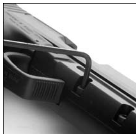
Fig. 31 Removing USP Match counterweight with 3 mm Allen wrench
