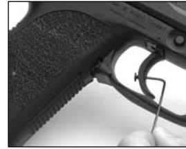
Fig. 27 Trigger stop adjustment with 1.5 mm Allen (hex) wrench
