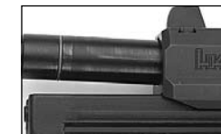
Fig. 31 O-ring shown on barrel
