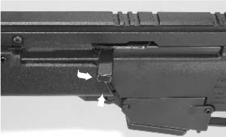
Fig. 24 Push cocking lever inwards (closing aid)
