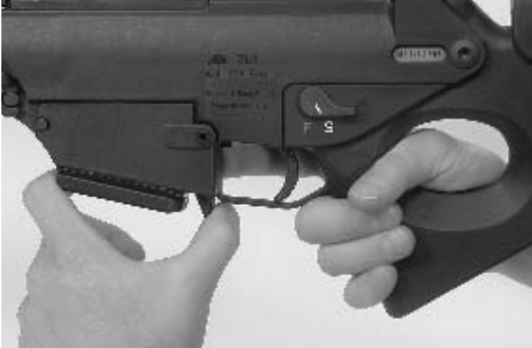
Fig. 23 Push magazine catch forwards
