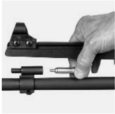
Fig. 29 Removal of gas piston
