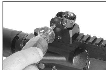
Fig. 77 Rotating the windage adjusting screw
