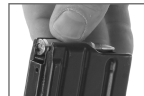
Fig. 67: Loading first round into magazine
