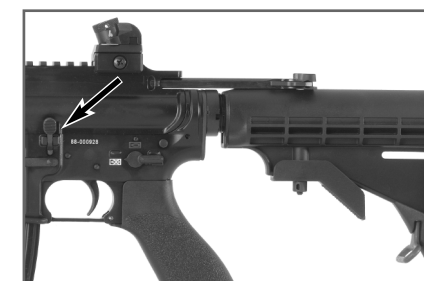
Fig. 13: Shows lower portion bolt catch depressed
