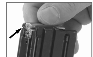
Fig. 69: Incorrect loading of cartridges (31 rounds)
