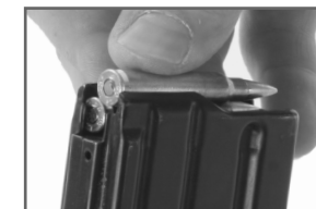
Fig. 68: Loading second round into magazine
