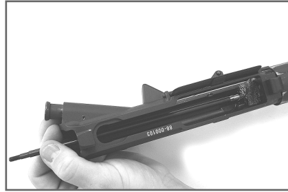
Fig. 57: Cleaning the Chamber
