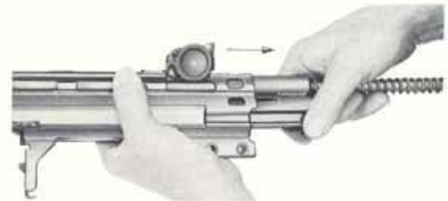
Fig. 34 Removal of bolt assembly
