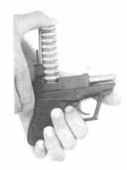
When loading an 11th round, press it down halfway through the magazine lips. Carefully let the slide forward about a 1/4" to pass the 10th round, and then let the slide go forward.
