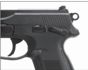
Hammer decocked for double-action firing
