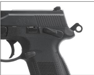
Hammer cocked for single-action firing
