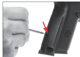
Use a small instrument to press the backstrap retainer.
