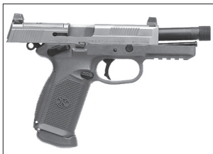
The slide locks to the rear after the last cartridge has been fired.
