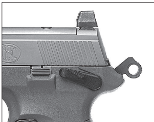
Hammer cocked for single-action firing
