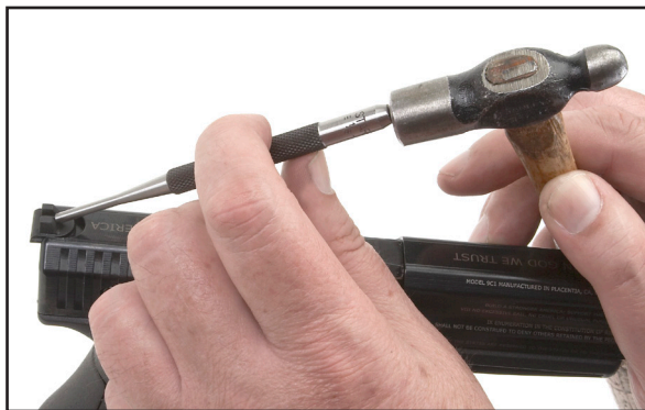
The rear sight can be removed by tapping on it rearward with a small punch.
