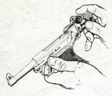
5. Toggle link and breechblock assembly can now be withdrawn from the rear of the receiver.
