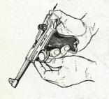
Push barrel with receiver assembly forward; this will enable the locking bolt to be removed.
