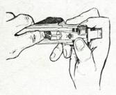
8. Push downwards with finger tip the sear, this allows the breechblock to close.
