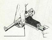
Check to ensure the pistol is unloaded. Push magazine catch and remove the magazine.
