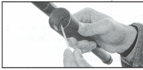
Fig 13: The two holes in the barrel gas porting ring which must remain open and clear for the shotgun to function properly. Make sure these two holes are cleaned after each use as
