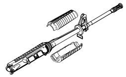
Remove the top hand protector and loosen the rear clamp screw (1). Install the upper portion RAS with the front locking spring tab under the handguard cap. Position the rear clamp over the gas tube and into the barrel nut. Tighten the clamp screw to secure the rear of the RAS. Slide the top hand protector onto the RAS from the rear. The lower portion of the RAS is assembled in the same manner.
