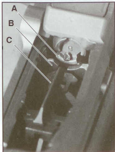
Fig. 4 – Bolt latched open.
