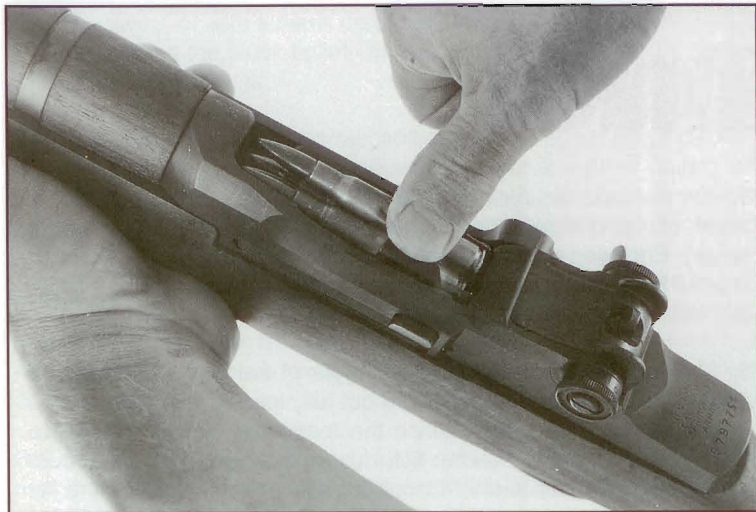
Fig. 3 – Push straight down to load a full clip into the rifle.
