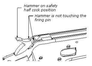
Hammer in safety position is strictly recommended when firing is not imminent and cartridge is chambered.
