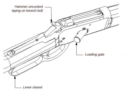
With the muzzle pointed in a safe direction, the lever must be completely closed to load the magazine. The hammer must not be cocked. With thumb securing hummer pull the trigger and slowly lower the hammer.
