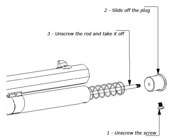
When the rod has been taken off, replace the plug in its seat. In Take Down version there are two screws to disassemble.
