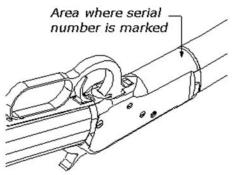
The serial number of the gun is visible under the receiver. It must not be removed or modified for any reason.
