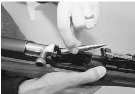
With the operating handle locked in its rearward position and the safety lever in the "ON" position, load rounds into the top of the magazine either manually (one at-a-time) or with the aid of a stripper clip.
