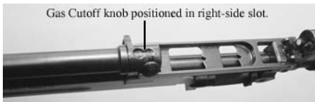
The Gas Cutoff knob must be set in the right-hand slot for the rifle to function. The left positions were used only when launching grenades.
