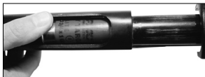
Loading a shell into the magazine when both the chamber and magazine are to be loaded.
