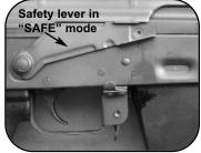
Safety lever in upper "SAFE" position. The lever is covering the stamped letter "S" on the receiver.
