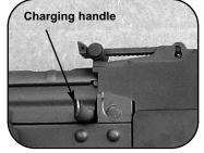
Pull back charging handle to load or eject a round from the chamber.
