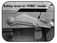
Safety lever in lower or "FIRE" position. Pulling the trigger when the safety lever is in the lower position will result in the rifle firing if there is a round in the chamber! Exercise extreme caution when handling the rifle in this condition.
