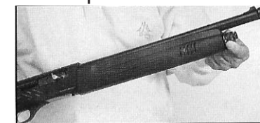
Fig. 5A: Screw on the forend cap so that the forend is held firmly in place. With the forend and the barrel in
