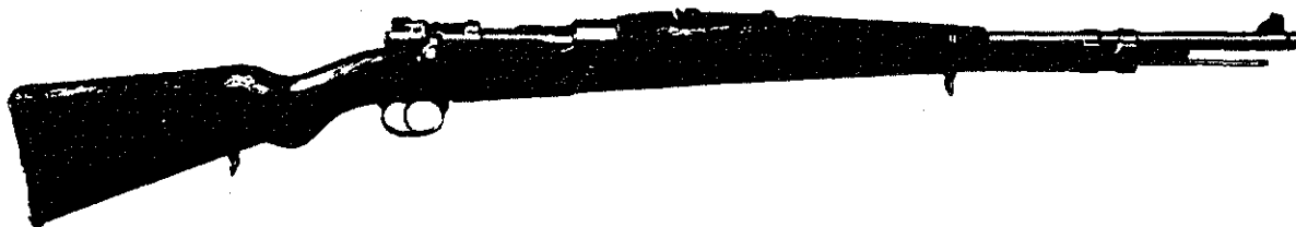
Right side view of the F. N. rifle (Mauser System)
