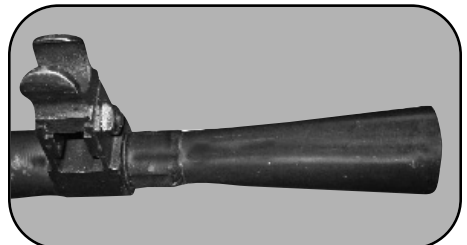
Flash hider installed on barrel.
