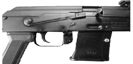
The loaded magazine is inserted into the pistol's magazine well by angling the magazine and inserting its flat-sided edge into the magazine well first, and then moving it into the well so that its other edge (containing a projection) locks into place in front of the trigger guard. Pull on the magazine slightly to ensure it is locked into position.
