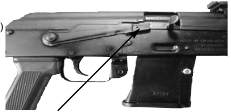
Safety Lever in upper or "SAFE" position. Lever is covering the imprinted letter "S" stamped into receiver.
