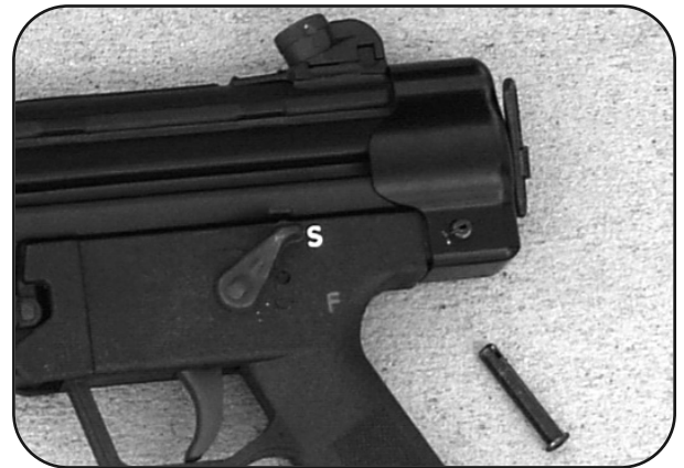
Figure 21 Remove the buttcap
