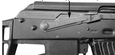
Safety Lever in "Safe" position. Lever is in upward position covering the stamped letter "S" on the receiver.
