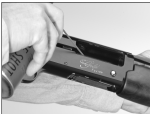
Place a drop of light gun oil inside the receiver on the rails.
