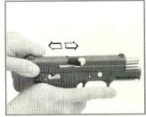
Being extremely careful not to touch the trigger, hold the pistol in your firing hand, point in a safe direction, pull the slide fully backwards with the other hand and then release the slide which returns under spring force.
