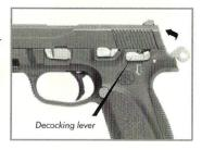
After this operation, the pistol can still be fired by pulling the trigger: firing will require a longer and stronger pull on the trigger.
