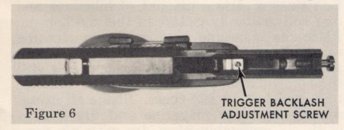
the frame. Turning the adjusting screw in a counter-clockwise direction increases backlash. Beyond a certain point, backlash can be reduced no more and further tightening of the backlash screw will only stiffen trigger pull, ultimately causing the trigger to become inoperative.
