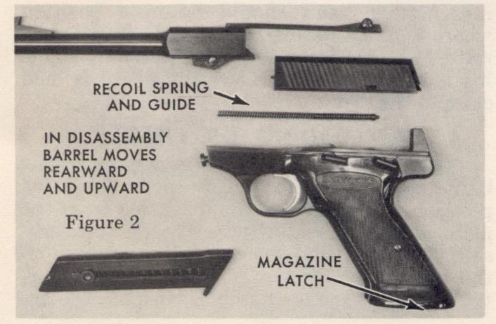
tion and chamber to be sure that a live cartridge is not remaining in the pistol. The stop open latch does not operate with the magazine removed unless the slide is locked into its rearward position manually or unless the magazine is removed after the last shot is fired, in which event the slide has already been locked rearward automatically.
