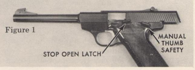
ure when on the range or while in storage. Also, since the slide stays open automatically after the last shot is fired, it is a signal the gun is empty (Fig. 1).
