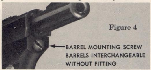
2. Located under the barrel on the front of the frame is a coin slotted barrel mounting screw. Using a screwdriver or a dime, loosen this screw until it becomes disengaged from the barrel (Fig. 4). It is unnecessary to remove the screw completely from the frame.
