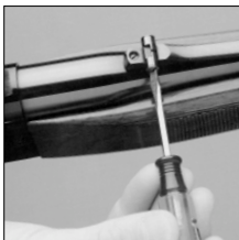
Horizontal Sight Adjustment
