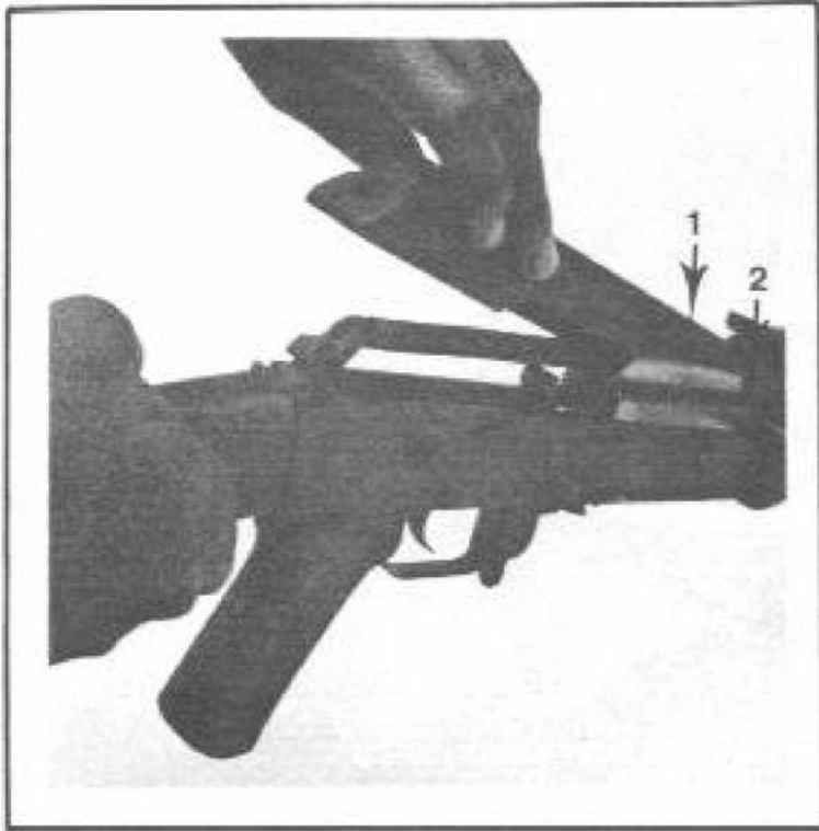
FIGURE 45. REPLACING BOLT COVER
