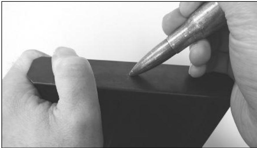
Fig. 15 Stripping The Magazine – Removing The Base Plate Stage 1
