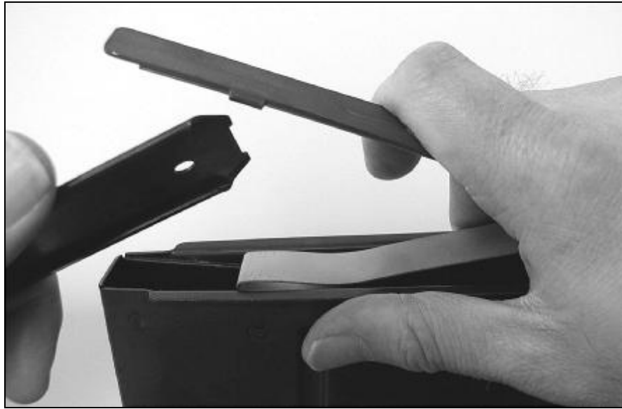
Fig. 17 Stripping The Magazine – Removing The Spring Assembly
