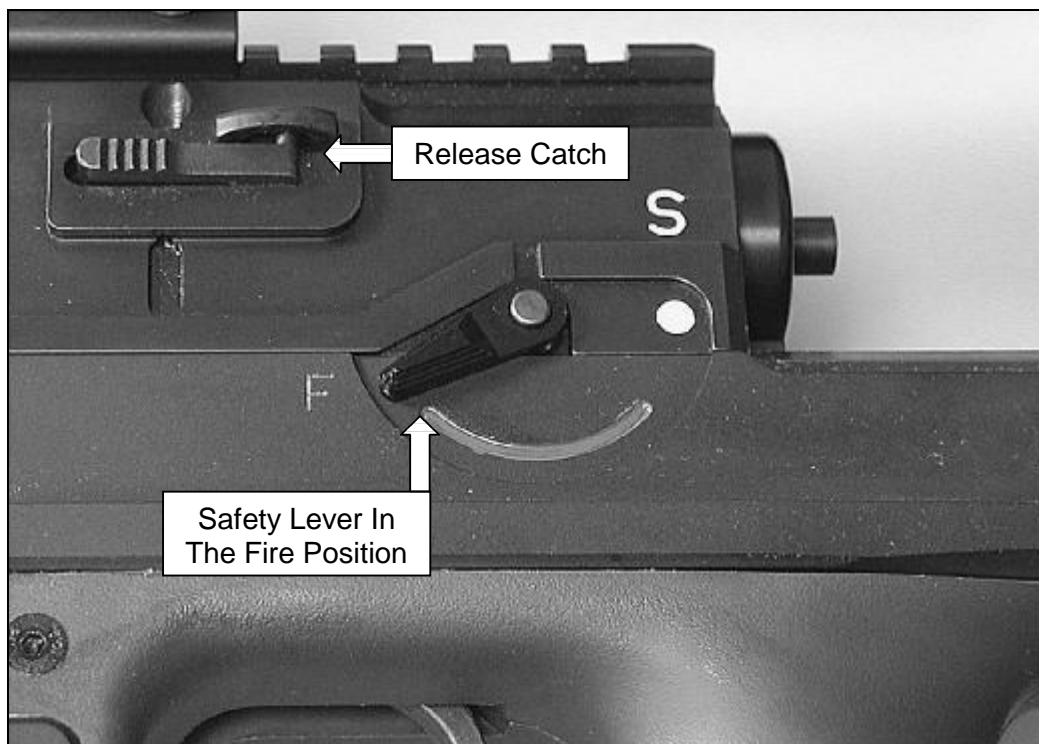
Fig. 09 Fitting & Removal Of The Bolt
