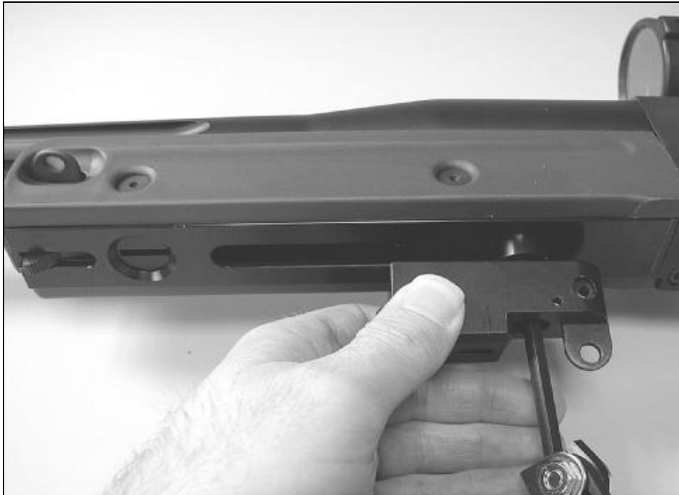
Fig. 06 Fitting & Removal Of The Hand Stop/Bipod Mount
