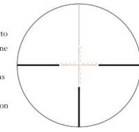
ensures that mrad specifications can be kept to the tightest tolerances possible. The fine center crosshair subtensions on the EBR-1 MRAD reticle were carefully chosen to provide the optimum balance between precision aiming and low light visibility.
